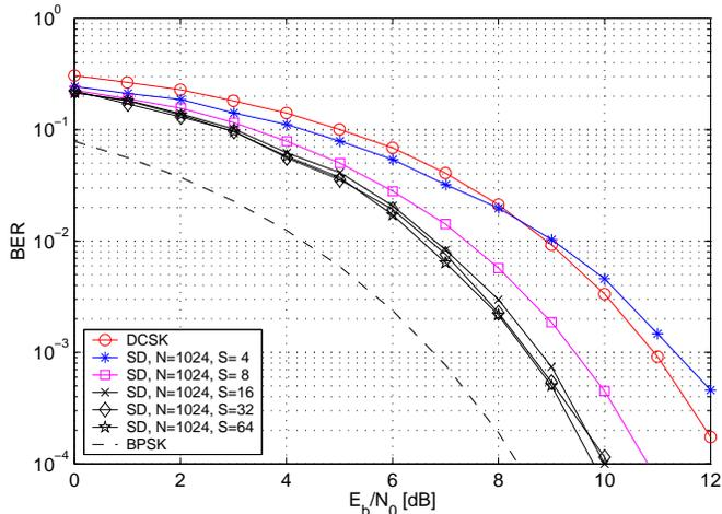
Fig. 5. BER performance: DCSK versus pseudo-chaotic modulation. Note the dependence on the number of states  $S$  in the Viterbi detector and the high error probability associated with the threshold discriminator (THR).
