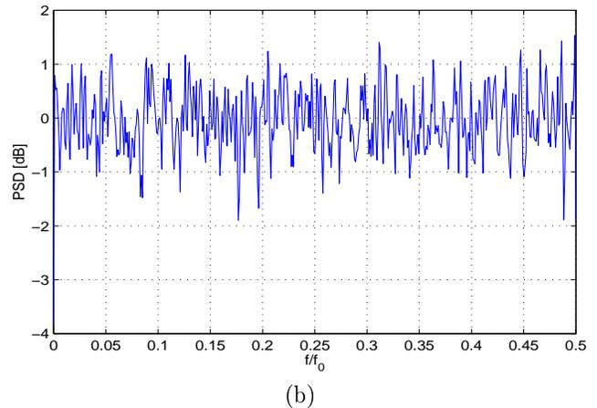
Fig. 4. (a) Transmitted SD-DCSK signal (for  $M = 10$ ) and (b) corresponding PSD (power spectral density). The plots refer to normalized time  $t/t_0$  and normalized frequency  $f/f_0$ , where  $t_0 = 1/f_0$  is the sampling period.
