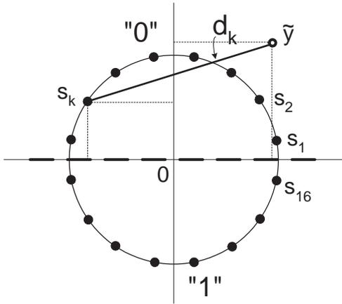
Fig. 3. Signal-space diagram for the SD-DCSK transmitted signal (for  $M = 4$ ) illustrating the geometrical meaning of the branch metric  $d_k$ . Note also that the arc  $[0, \pi)$  is associated with the symbol "0", while  $[\pi, 2\pi)$  corresponds to the symbol "1".
