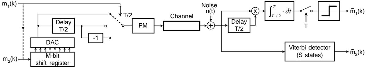
Fig. 1. Block diagram of the SD-DCSK scheme. For forward error-correction applications:  $m_2(k) \equiv m_1(k)$ .
