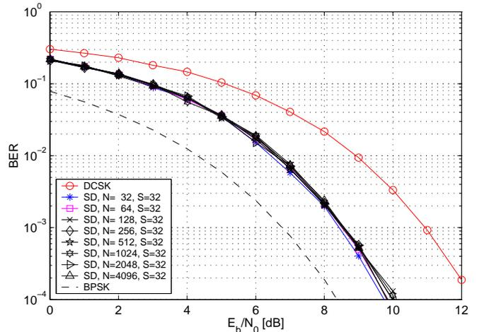
Fig. 6. BER dependence on the number  $N$  of transmitter levels, for a fixed complexity ( $S = 32$ ) of the Viterbi detector. Note that the performance is basically independent from the number of transmitter levels.
