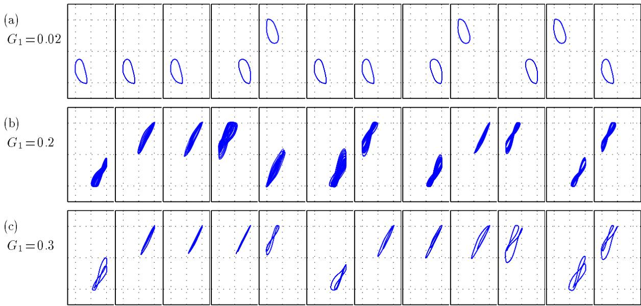
**Figure 3:** Synchronization of the neighboring cells for the steady-state behavior of the lattice composed of  $n = 12$  chaotic cells for different coupling conductance  $G_1$ . In the  $i$ th column the projection of the steady-state onto the  $z_i, z_{i-1}$  plane is shown ( $z_0 = z_{12}$ ),  $z_i, z_{i-1} \in [-3, 3]$
