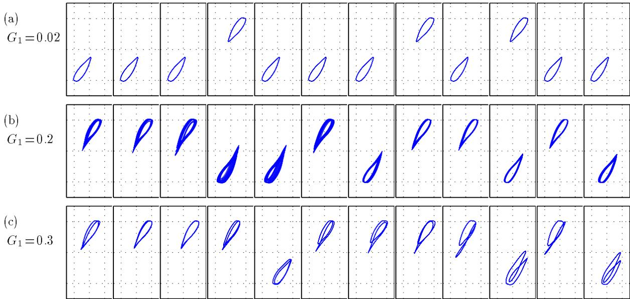
**Figure 1:** Steady state behavior of the lattice composed of  $n = 12$  chaotic cells for different coupling conductance  $G_1$ . The projection of attractor onto the  $y_i, z_i$  plane for cells  $i = 1, \dots, 12$  is shown,  $y_i, z_i \in [-3, 3]$
