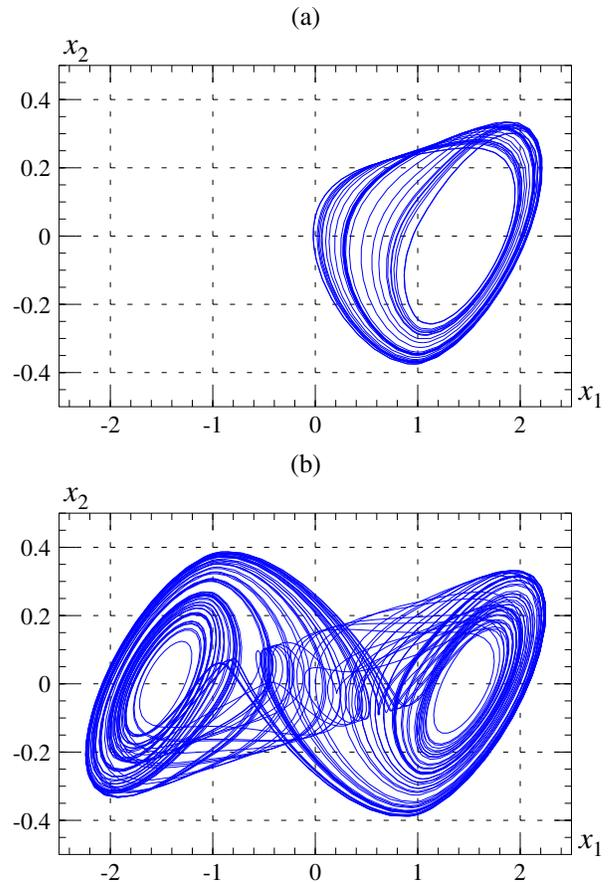
Fig. 1. Computer simulations of Chua's circuit. (a) Roessler-type attractor for  $C_2 = 7.65$ , (b) double-scroll attractor for  $C_2 = 9.3515$
