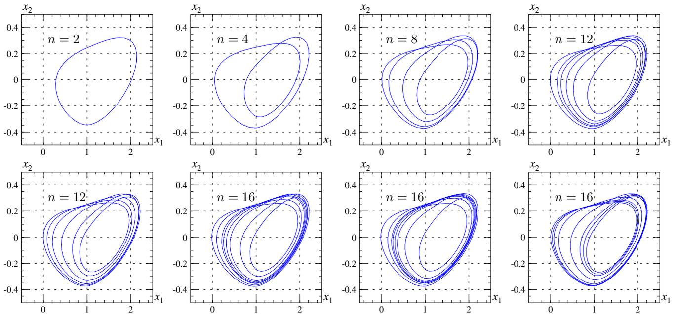
Fig. 3. Short periodic orbits of the Chua's circuit,  $n$  is the number of intersections with  $\Sigma$
