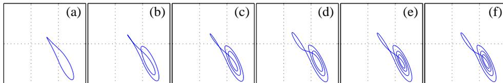
Figure 5: Periodic orbits for the Chua's circuit, projection to the plane  $(x_1, x_2)$ , (a) period-2 orbit, (b)–(f) period-4 orbits of the Poincaré map
