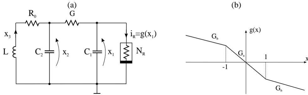
Figure 1: Electronic circuit (a) and characteristics of the nonlinear resistor (b)
