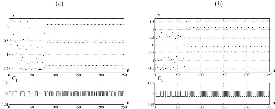
Figure 2: Stabilization of periodic orbits of Chua's circuit using the bang-bang control method, (a) periodic orbit  $\gamma_{1,0}$ ,  $n = 3$ ,  $\Delta_p = 0.002$ , (b) periodic orbit  $\gamma_{2,2}$ ,  $n = 8$ ,  $\Delta_p = 0.0025$
