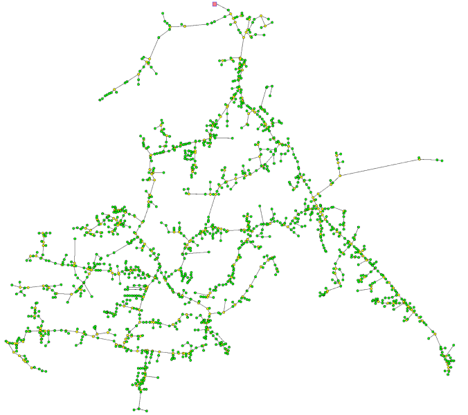
Fig. 2. Structure of the IEEE 8500 Node Test Feeder, the number of nodes is reduced to n = 2250 by removing single-child distribution nodes.
