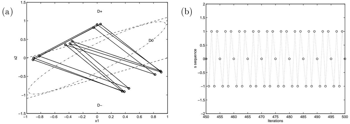
Figure 7:  $r = 1/15$ ,  $x(0) = (0.85, -0.4)^T$ ,  $s = (-+-+0)$ ,  $L = 5$ , (a) The trajectory travels in  $D_0$ ,  $D_+$  and  $D_-$  periodically with period  $3 \times 5 = 15$ , (b) The  $s$  sequence of the last 50 iterations.
