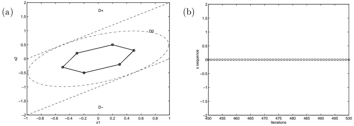
Figure 1:  $r = 1/6$ ,  $x(0) = (0.5, 0.3)^T$ ,  $s = (0)$ ,  $L = 1$ , (a) The trajectory travels on an ellipse in  $D_0$  with period 6, (b) The  $s$  sequence of the last 50 iterations.
