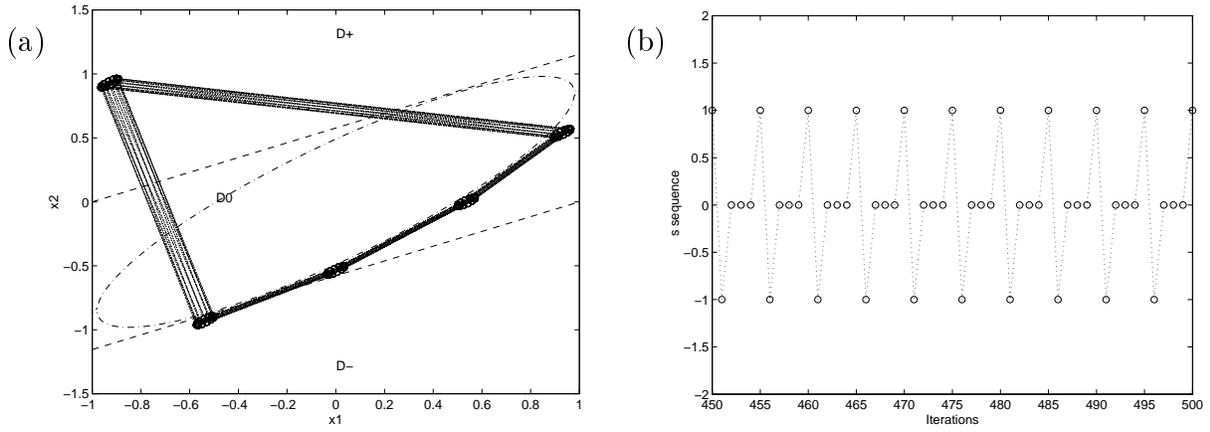
Figure 3:  $r = 1/12$ ,  $x(0) = (0.9, 0.5)^T$ ,  $s = (+-000)$ ,  $L = 5$ , (a) The trajectory travels in  $D_0$ ,  $D_+$  and  $D_-$  periodically with period  $5 \times 12 = 60$ , (b) The  $s$  sequence of the last 50 iterations.
