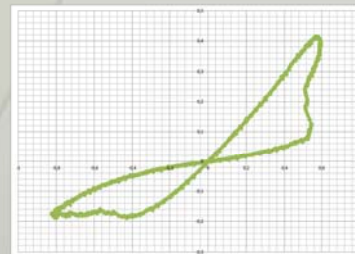
U-I: Amplitude=1V, Frequency=500Hz, Offset=0.0V
