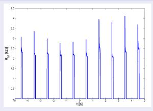
When the input signal is positive then the resistance of the element decreases. This behavior corresponds to the OFF-ON switching in which the memristor's resistance changes from a high value to a low value.
