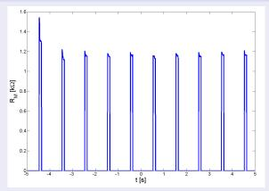
The switching takes place during the first two pulses and then the resistance stabilizes. The final value of the resistance  $R_{\rm M} \approx 1.2 \ \mathrm{k}\Omega$  is approximately two times smaller than in the first experiment ( $R_{\rm M} \approx 2.5 \ \mathrm{k}\Omega$  for  $U_{\rm IN} = 0.5 \ \mathrm{V}$ ).
