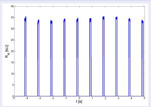
Applying the negative voltage  $U_{\rm IN}=-0.5~{\rm V}$  causes an almost immediate switching to high resistance state. The ON-OFF and OFF-ON switchings take place at different levels of the absolute value of the input signal.
