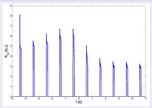
During the first four pulses the value of  $R_{\rm M}$  increases. For the remaining pulses the resistance decreases, as expected.
