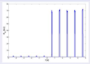
The switching occurs during the sixteenth voltage pulse. The memristor resistance changes to a much higher level  $R_{\rm M}\approx 70~{\rm k}\Omega$  than in the case  $U_{\rm IN}=-0.5~{\rm V}.$
