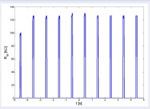
The ON-OFF switching takes place much faster—already during the first pulse the resistance reaches  $100~k\Omega$  and after the second pulse the resistance stabilizes around  $125~k\Omega.$
