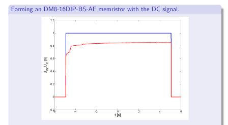
Input and output voltages versus time. Red line indicates output voltage  $U_{\rm R}$ . This experiment was repeated three more times, after which the resistance stabilizes.
