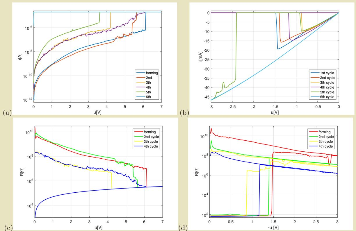
**Figure 2:** DC forcing - characteristics of switching process on the i-v plain (a,b). The device resistance changes during the switching process (c,d). Characteristics (a,c) presents the setting process of the device, while (b,d) resetting. Switchings appear at different non-repeatable voltage levels
