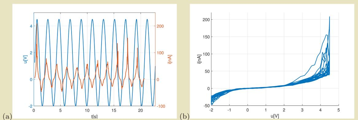
**Figure 3:** Sinusoidal responses. a) - time series of the applied voltage and responded current, b) i-v plot of the sinusoidal respond. When sinusoidal forcing is applied hysteric behaviour becomes visible.
