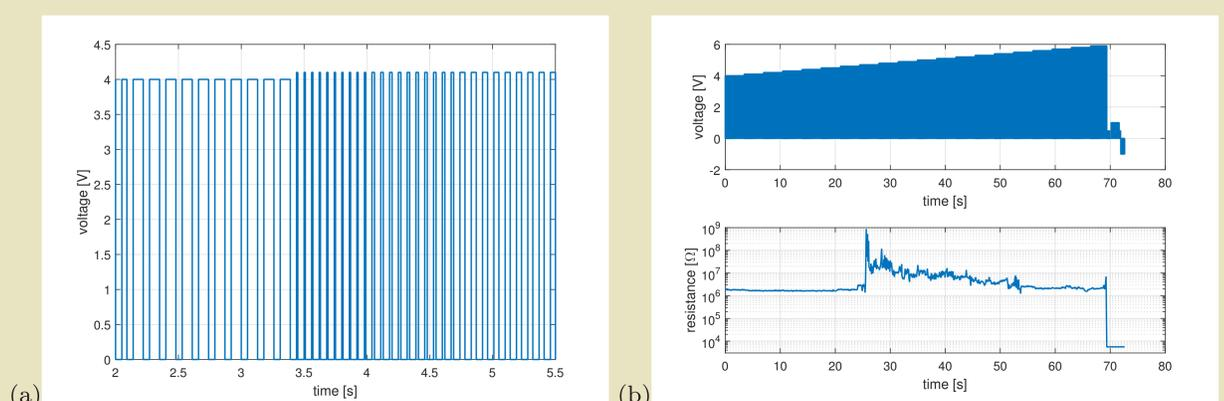
**Figure 4:** Programming the memory cell using pulses. a) the voltage pulses that were used to set the device. Both the pulses width and the amplitude were varied. b) the process of setting the device. Graph presents the applied voltage pulses series and the resistance of the tested device.
